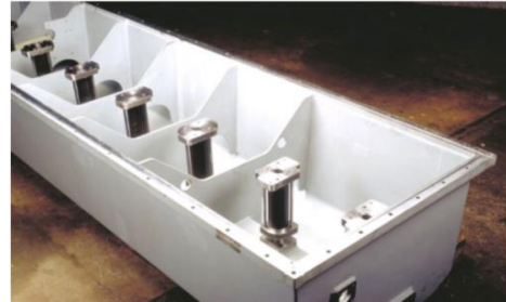
Fig: Oil sump
