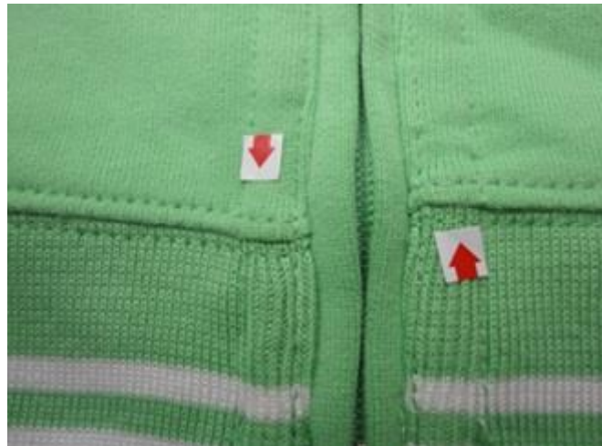
Fig3.10.6: Seams not aligned at crossing of seams
