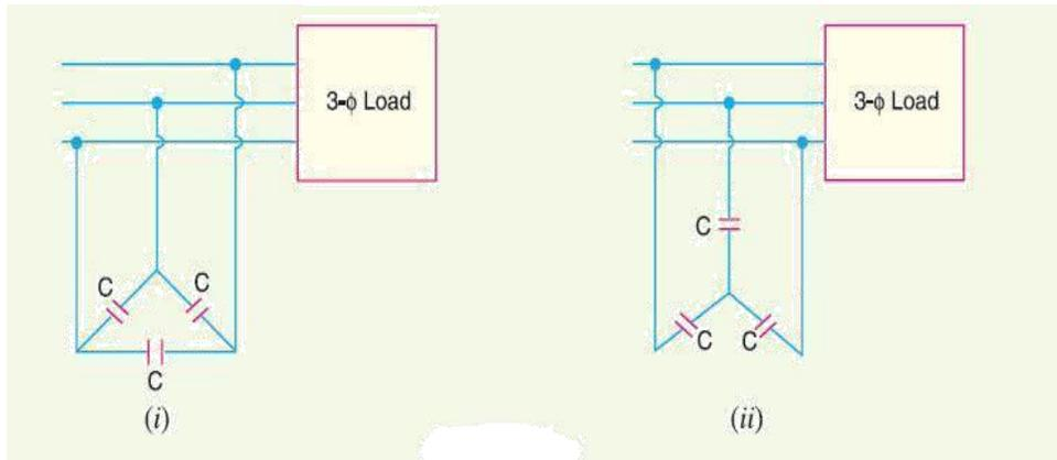
**Figure 6.3: Static Capacitor**
