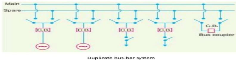
Figure 4.3 Double Bus-Bar Arrangement
