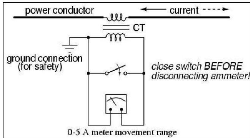
Figure 3.2: Simple Connection of CT
