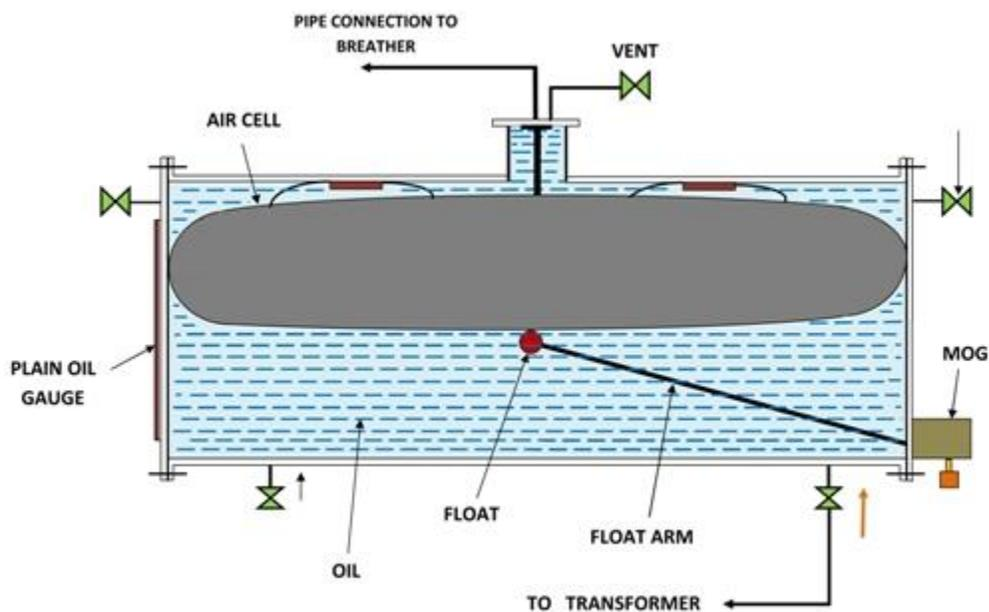
Figure 3.10: Conservator of Transformer
