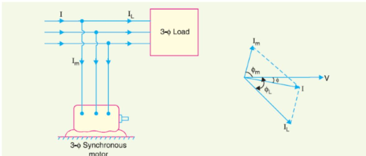
**Figure 6.4 Synchronous Condenser with Load of Motor**
