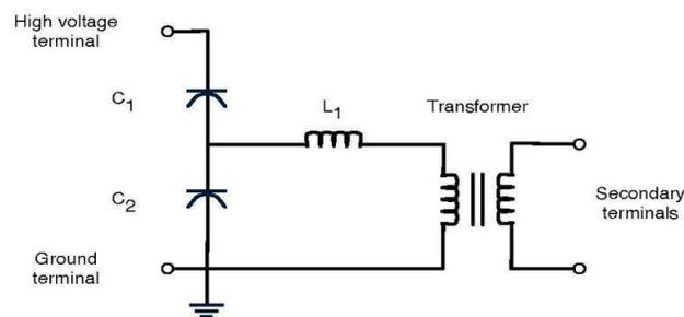
**Figure 3.14: Capacitor Voltage Transformer Diagram**
