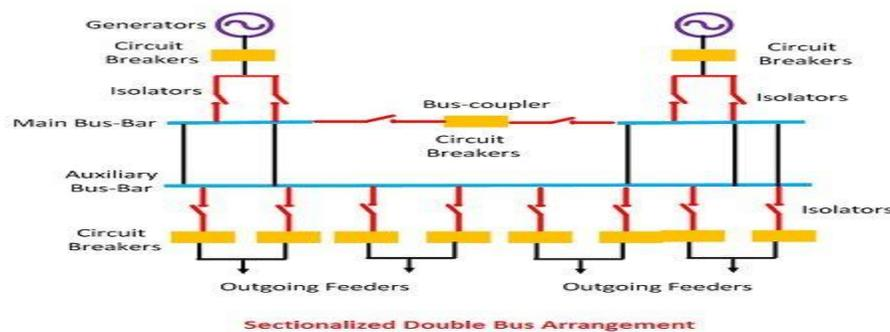
Figure 4.4: Double bus-bar with sectionalized
