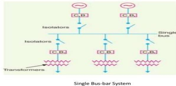
**Figure: 4.1 Single Bus-Bar Arrangement**
