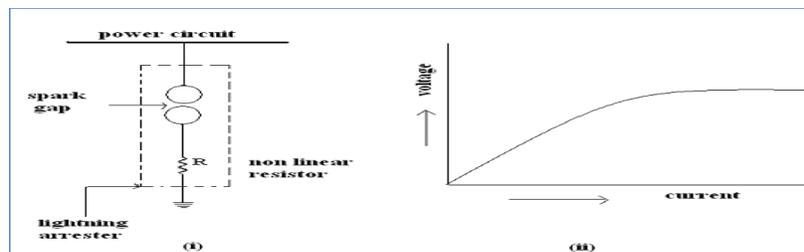
**Figure 3.12 Lightning Arrester**
