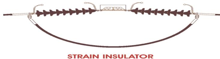
Figure 5.6: Strain Insulator
