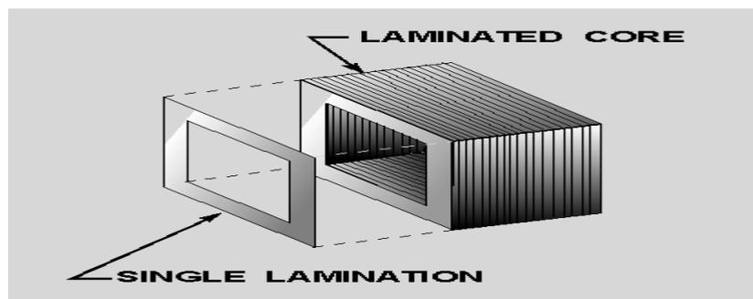
**Figure3.9: Laminated Core of Transformer**
