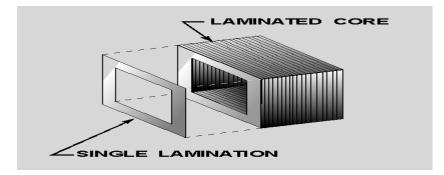
Figure 3.9: Laminated Core of Transformer
