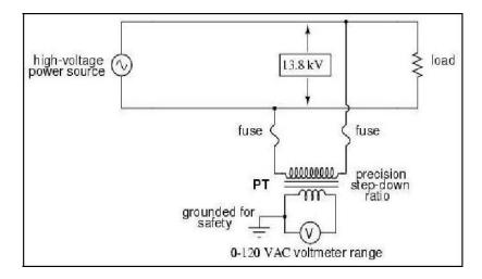
Figure 3.4: Simple Connection Diagram of Voltage Transformer
