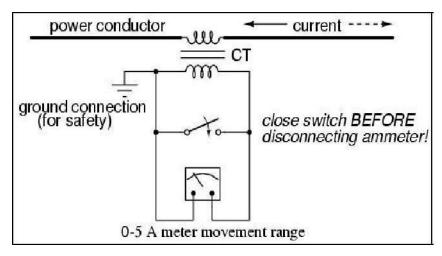
Figure 3.2: Simple Connection of CT
