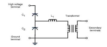
Figure 3.14: Capacitor Voltage Transformer Diagram
