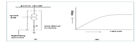
**Figure 3.12 Lightening Arrester**
