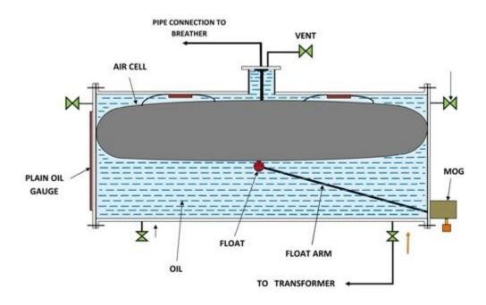
Figure 3.10: Conservator of Transformer
