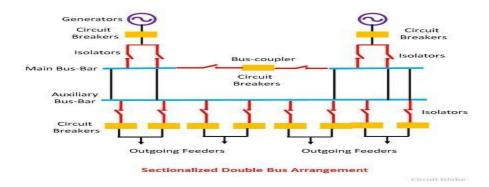
Figure 4.4: Double bus-bar with sectionalized
