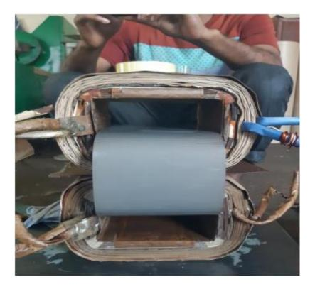
Figure 5.8: Transformer repairing in workshop
