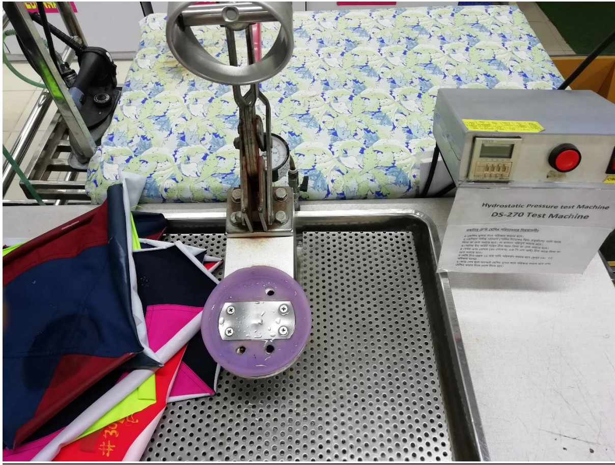
Figure No 14: Hydrostatic Pressure Test Machine.
