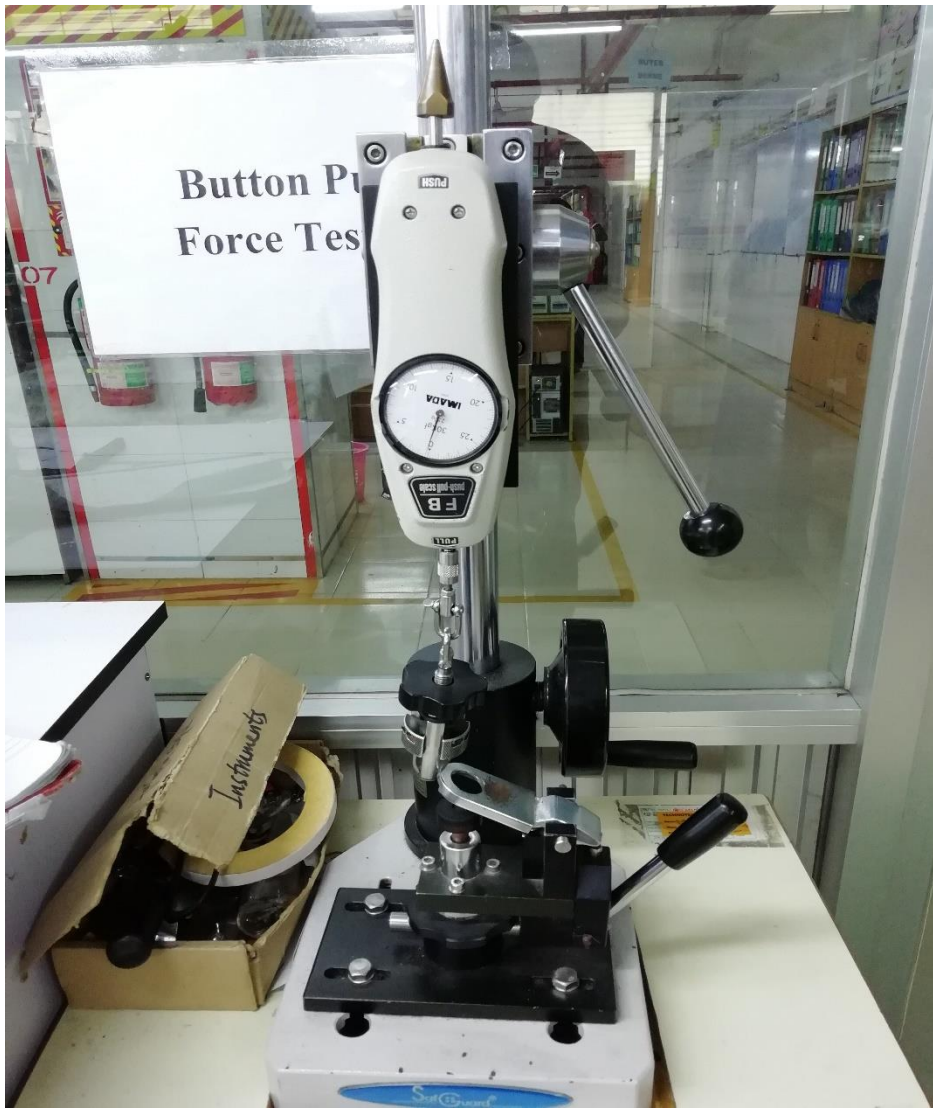
Figure No 12: Button Pull Force Test.
