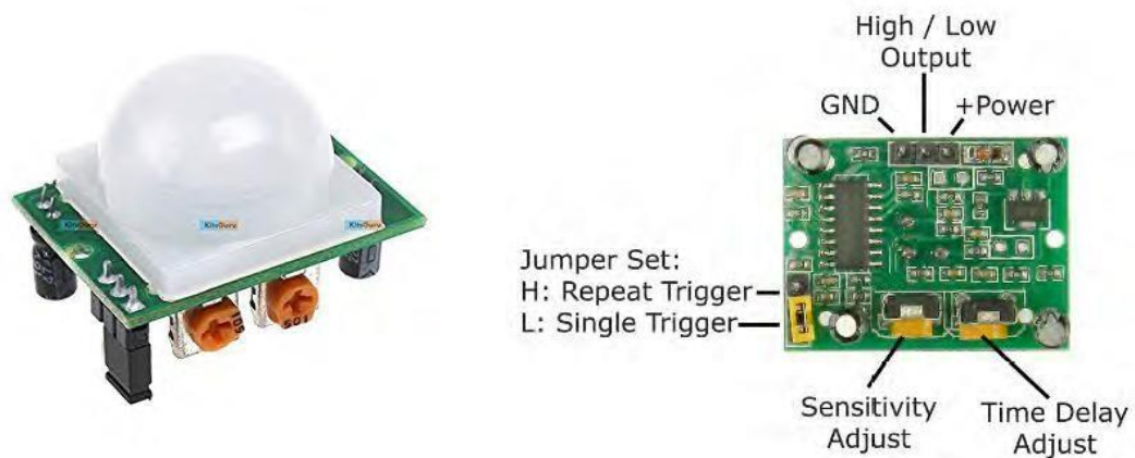
Figure 3.5: (a) PIR Motion Detector (Top view). (b) PIR Motion Detector (bottom view).
