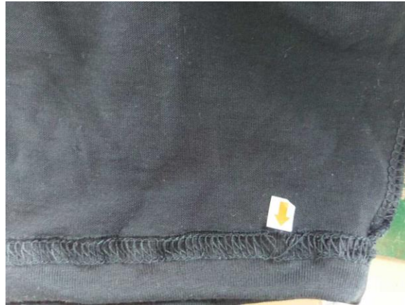
Figure 20: Tension lose loop
