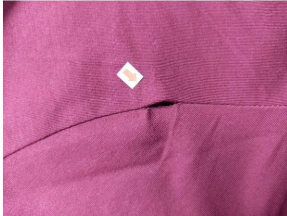
Figure 24: Arm hole joint problem
