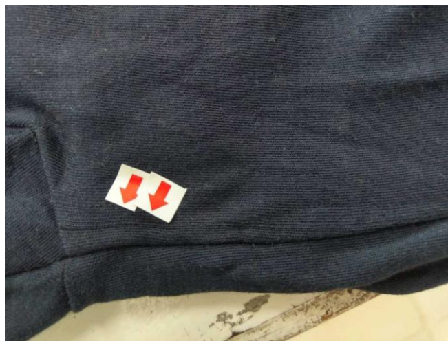
Figure 12: Yarn missing Fabric Fault
