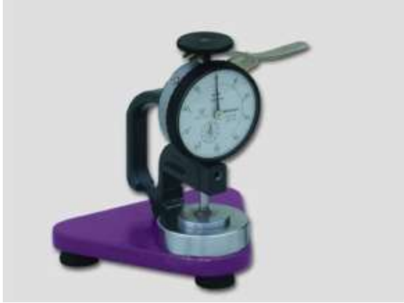
Fig: 3.3 Mag Ana thickness tester
