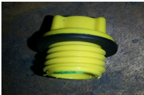
Figure 3.17: Vent cap of battery
