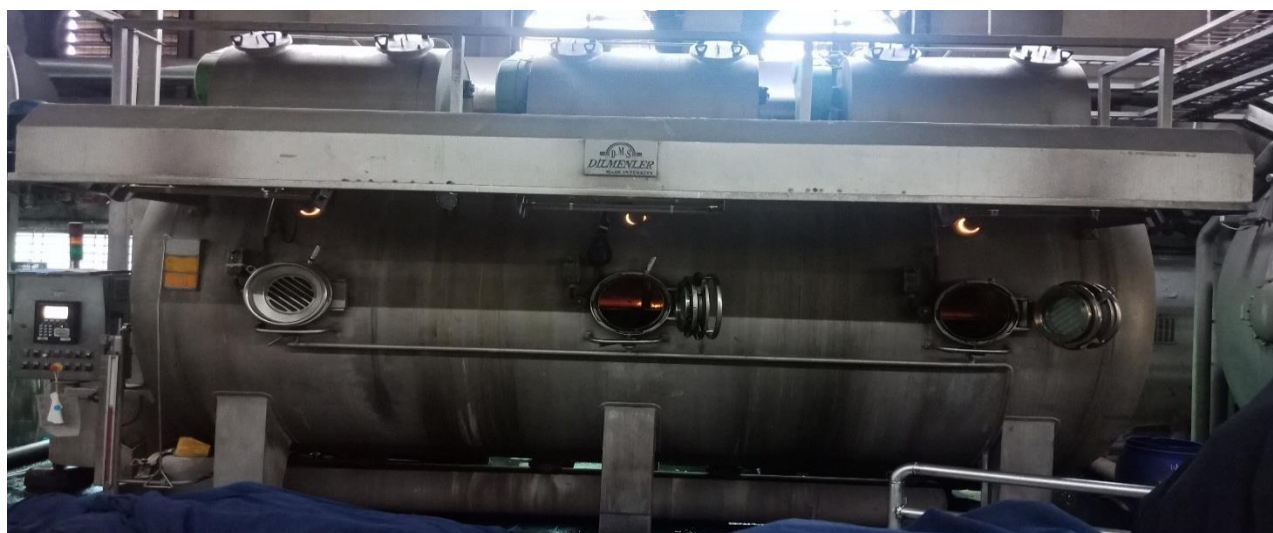
Figure: Winch Dyeing M/C
