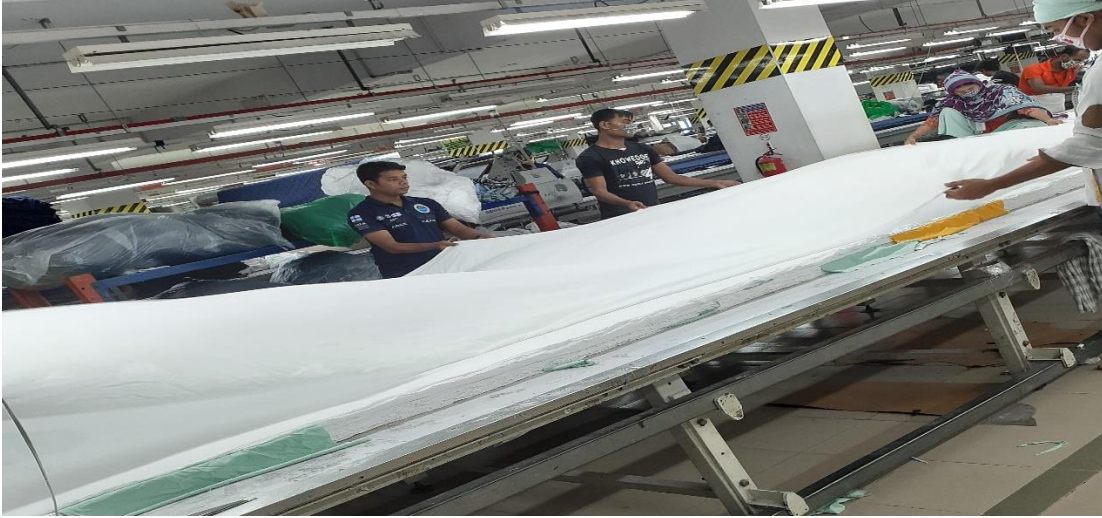
Figure 5.4: Manual fabric spreading.
