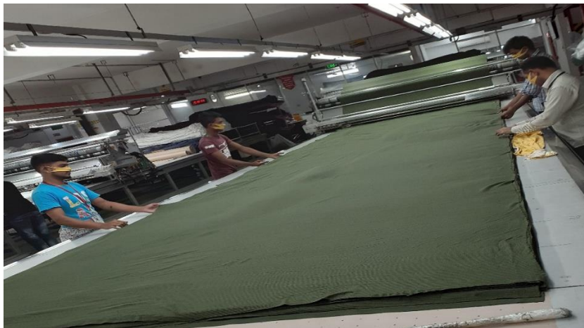
Figure 5.6: Automatic fabric spreading of 2 nd type of fabric lay
