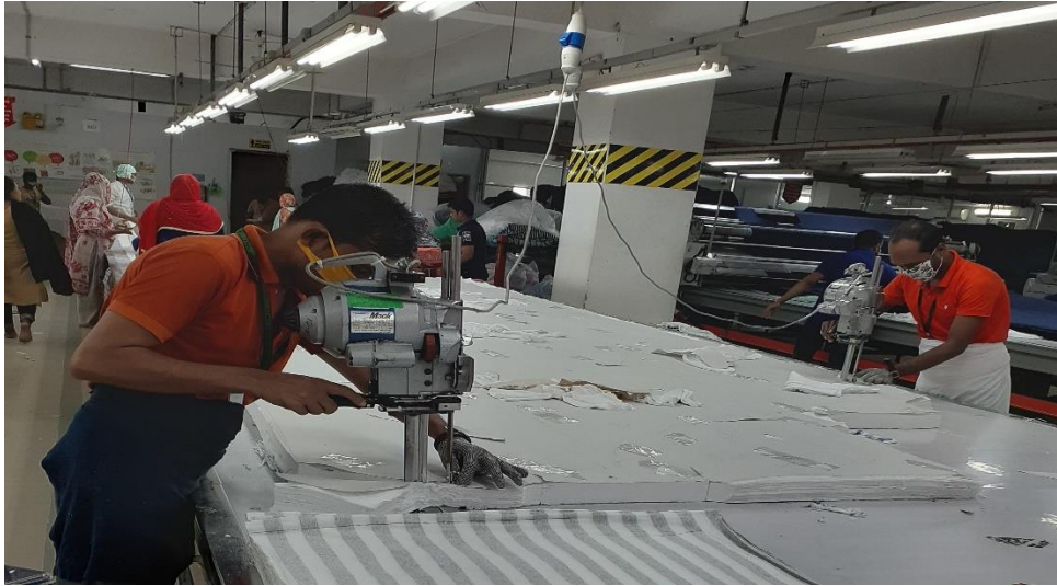
Figure 5.7: Manual fabric lay cutting method
