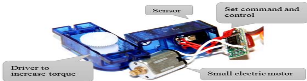
Fig 3.7 Physical Construction of Servo SG-90
