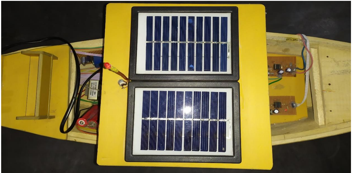
Figure 5.3: Solar panel day mode (charging)
