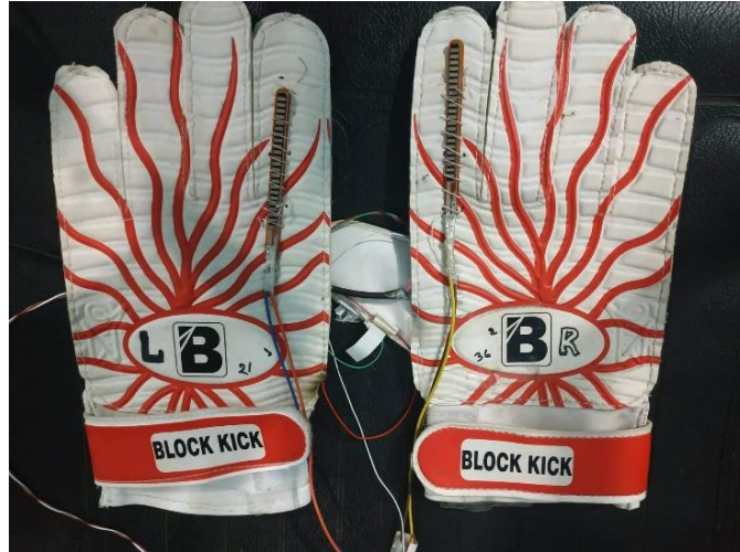
Figure 5.2: Installed Flex Sensors.
