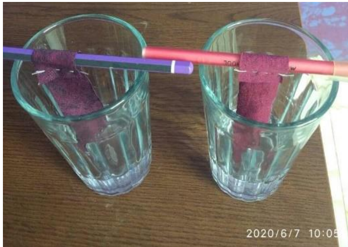
Figure 10: Vertical wicking test of Sangria colored fabric.
