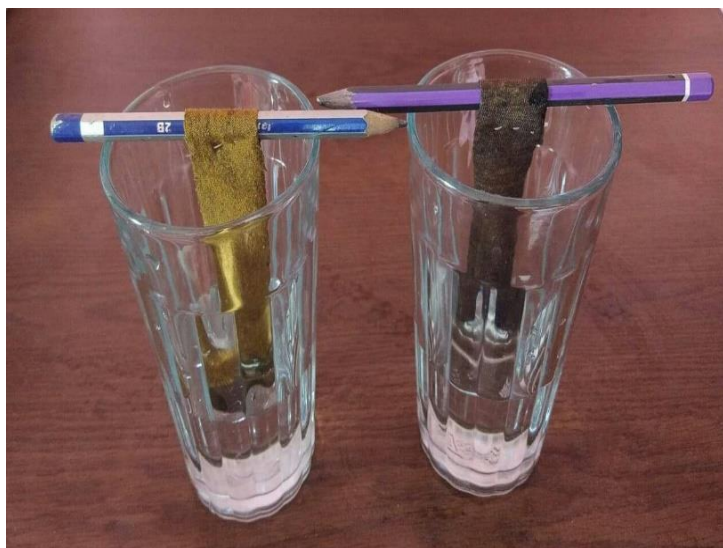
Figure 11: Vertical wicking test of Thai Curry colored fabric.
