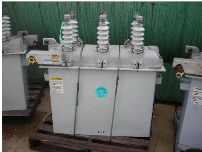
Fig 3.20: Oil Circuit Recloser
