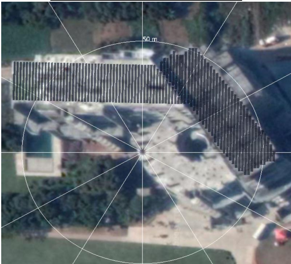
Figure 3.3: Solar Panel Design in AB-04 Roof Top
