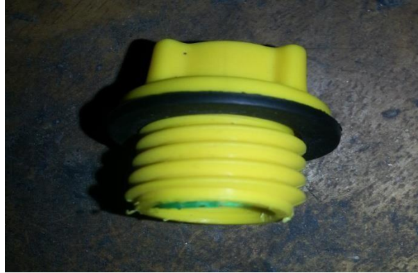
Figure 2.17: Vent cap of the battery
