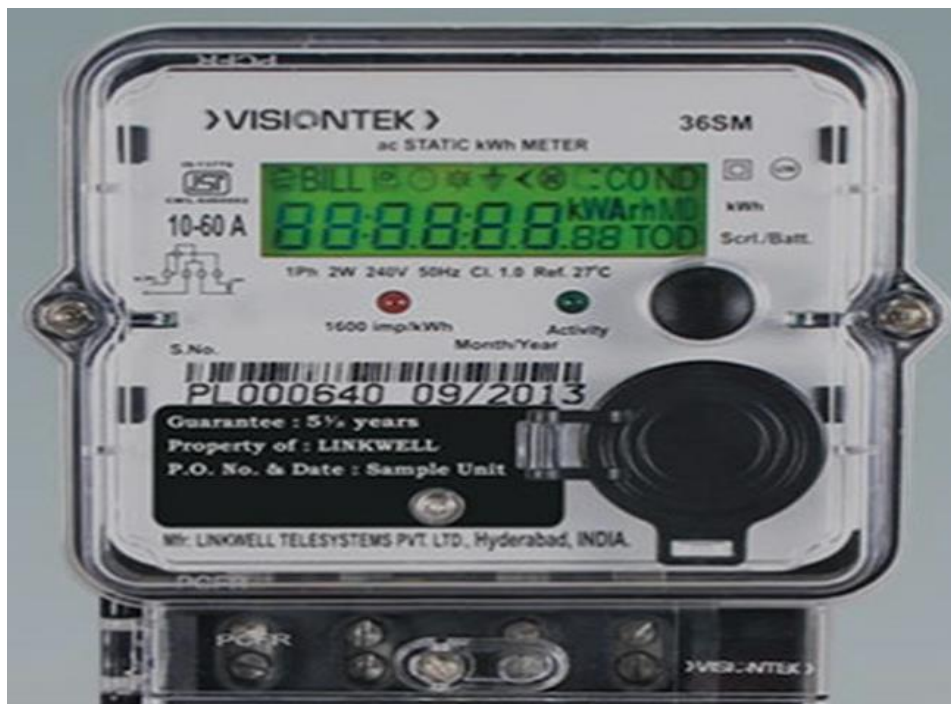
Figure 2.1: The electronic energy meter is only displaying a replica of the EEM. This receiver is a handheld device or radio base network installed in a mobile car for the collection and transfer of energy consumption data, through a wireless means such as ZigBee Zivic et al (2016a).
