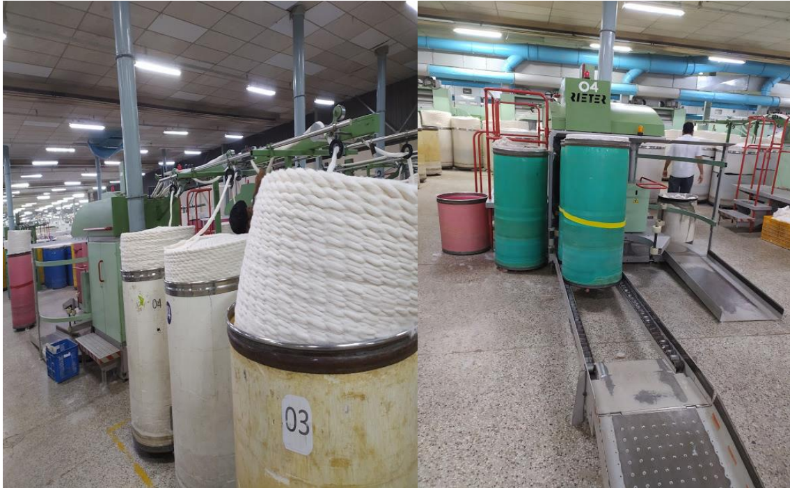
Figure 4 Breaker draw frame
