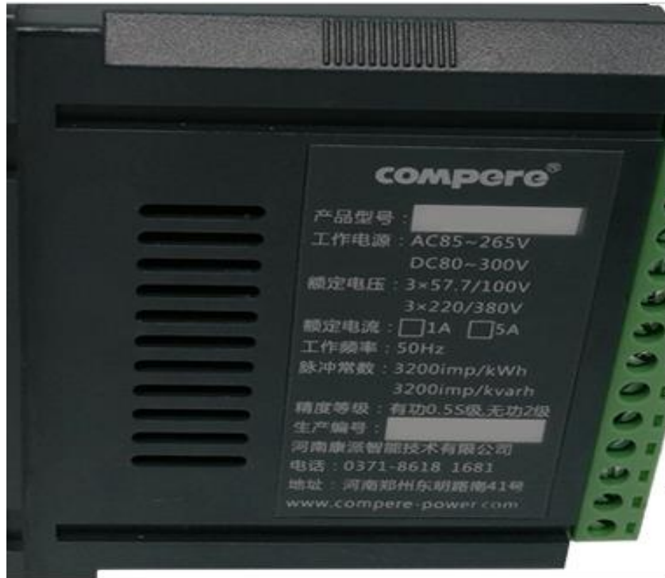
Fig 6.2: Rating of Four Quadrant Energy Meter
