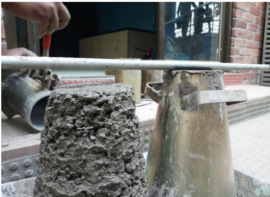
Figure 12: Slump Value Test
