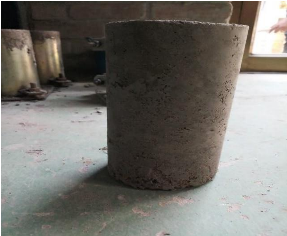
Figure 15: A complete cylinder for strength test
