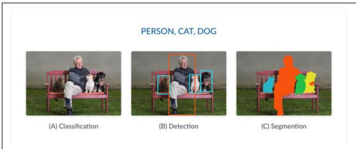
Figure 2.1.3.6: Classification, object detection & segmentation
