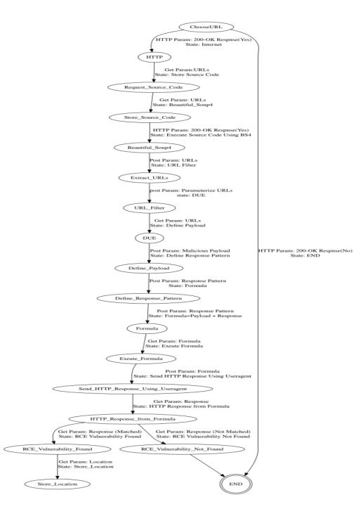
Figure 2: RCE Finite State Machine
