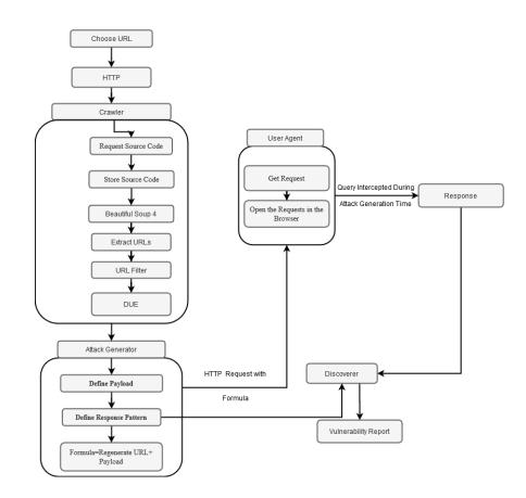
Figure 1: System Architecture of RCE Detection Model
