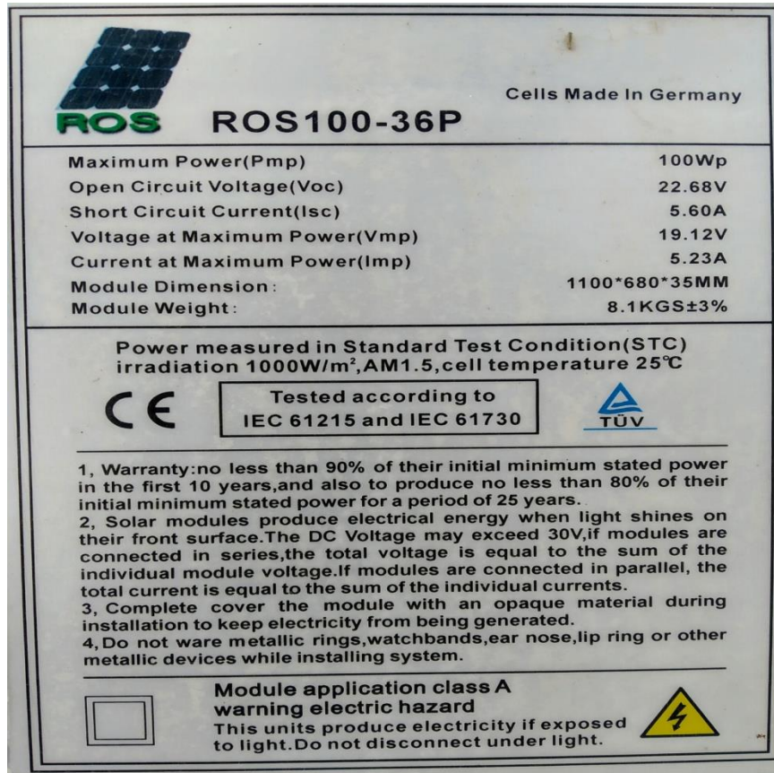
Figure 3.5 Electrical Specifications of 100W
