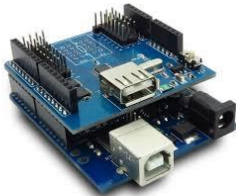
Figure 6.2.1: Arduino UNO & Arduino Host Shield
