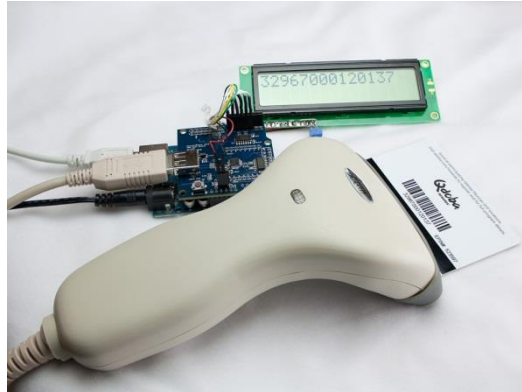
Figure 6.2.2: Arduino Host Shield & Barcode Scanner
