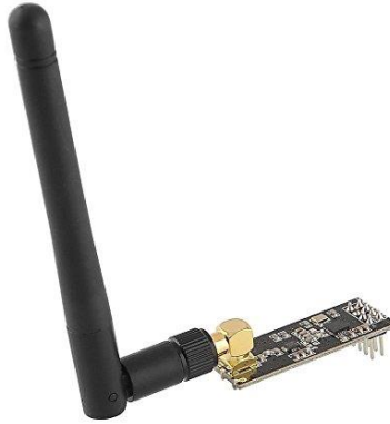
Figure 4.1.4: nRF24L01 Wireless Module with Antenna
