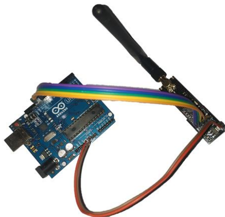
Figure 6.2.5: Arduino UNO & nRF24L01 & nRF24L01 Base
