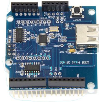
Figure 4.1.2: Arduino UNO USB Shield
