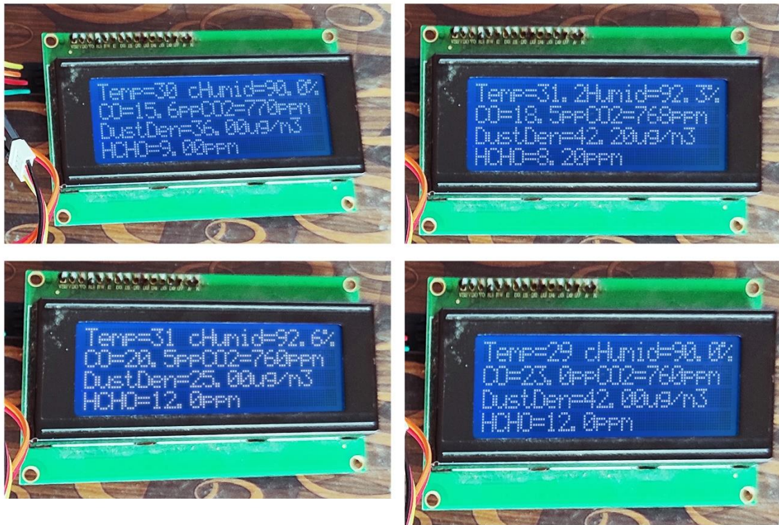
Figure 4.1: Real time contaminant measurement showed in LCD
