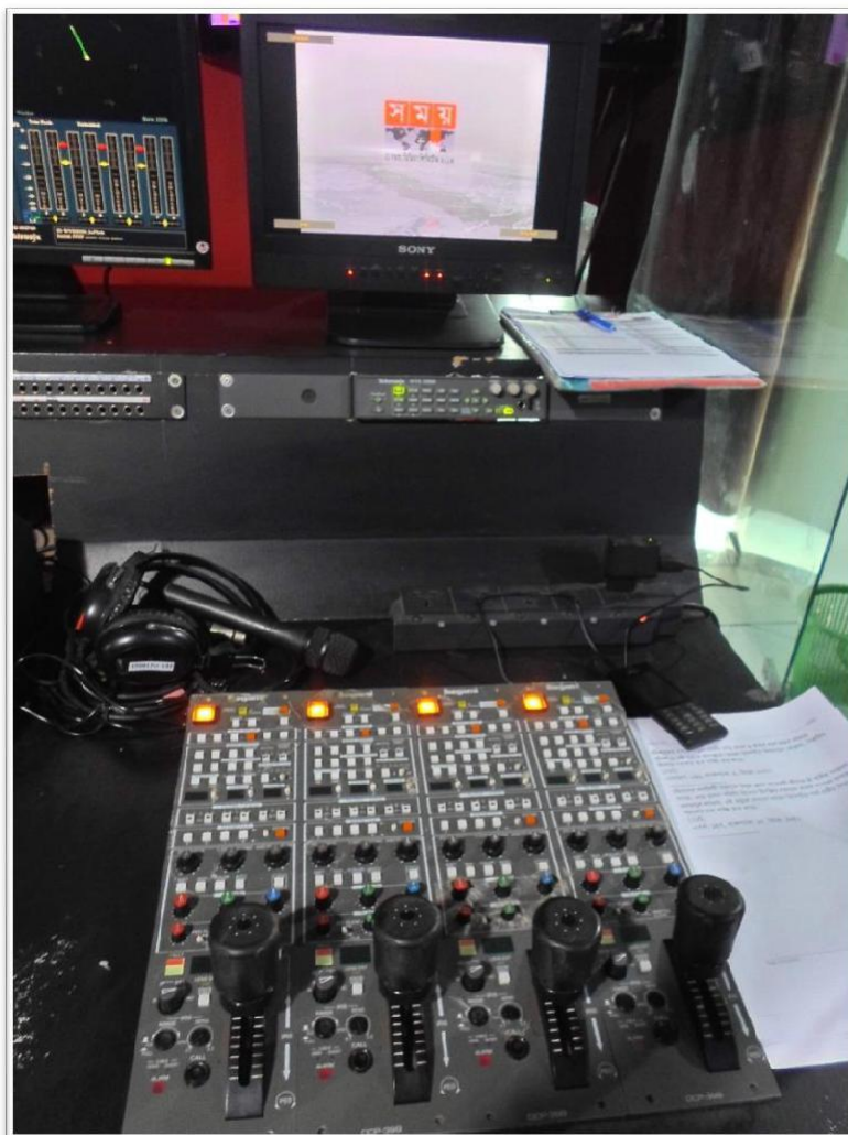
Figure 2.16 - Camera Control Unit
