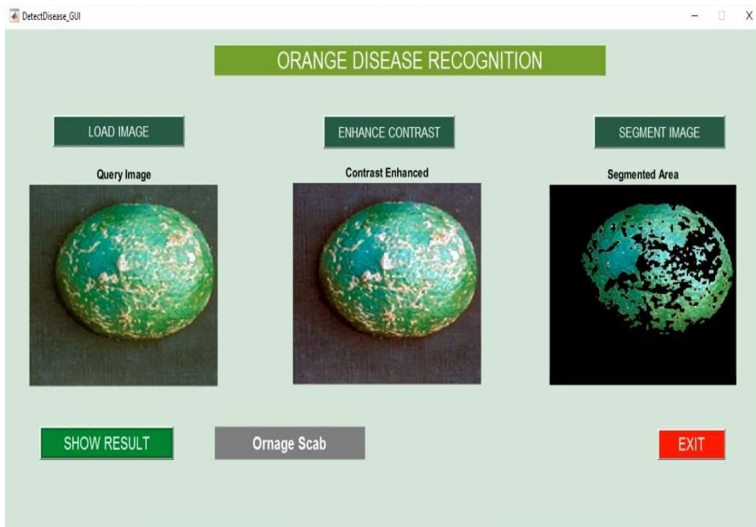
Figure 4.5: Classification result shown in the GUI for Orange Scab Disease
