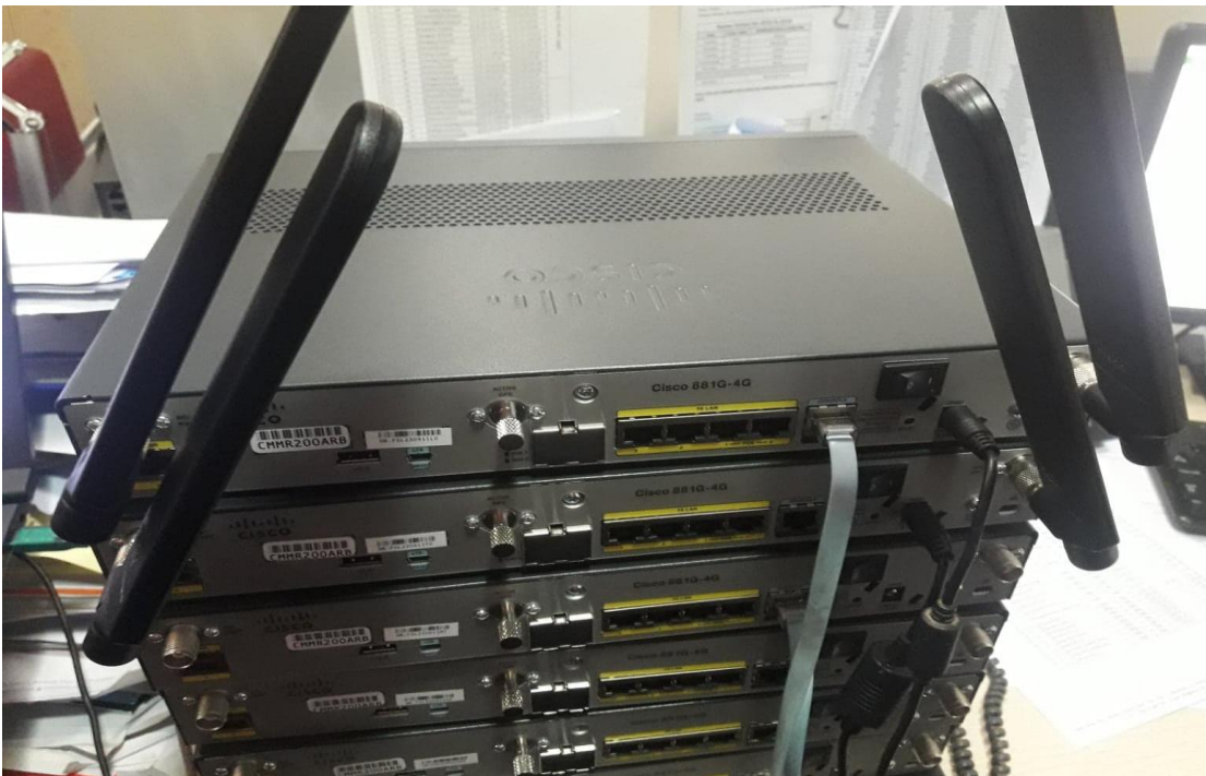
Fig 2.10: CISCO 881G-4G GSM based Router
