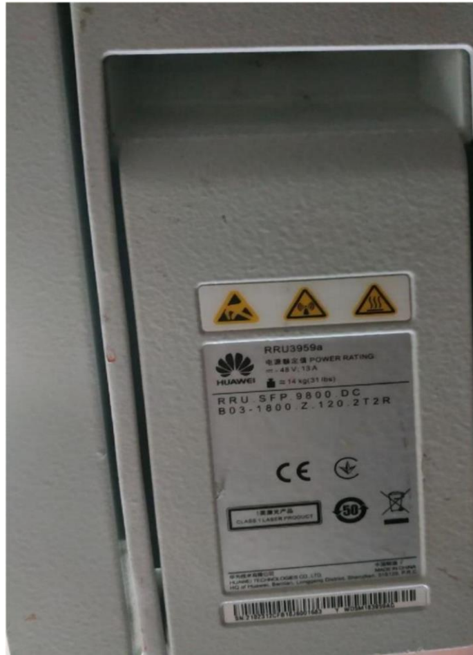
Fig-4.11: Remote Radio Unit (RRU)
