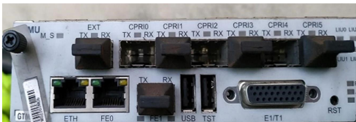
Fig-5.3: GTMU (GSM Transmission & Management Unit for BBU)
