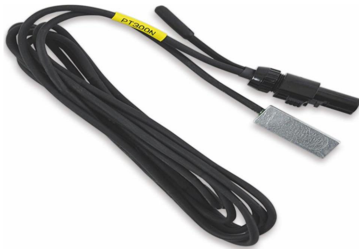
Figure 4.6: Cell Temperature Measurement
