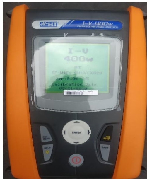
Figure 4.5: Photovoltaic Panel Analyzer (I-V 400W)
