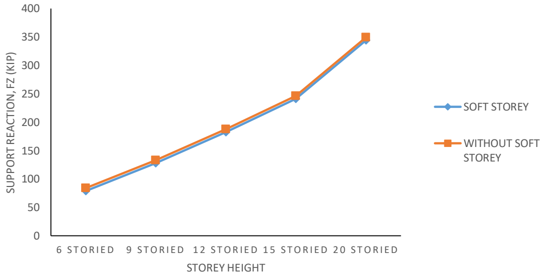
Figure 4.2(b): Comparison of Support Reaction for (-W x ) Combination DCON4
