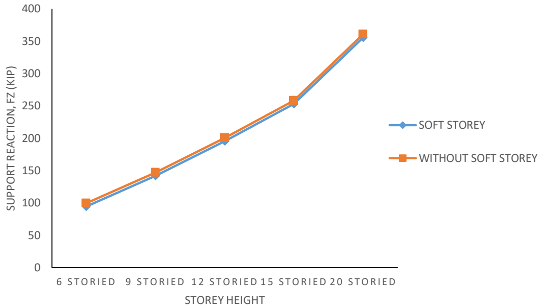
Figure 4.3(b): Comparison of Support Reaction for (-EQx) Combination DCON16
