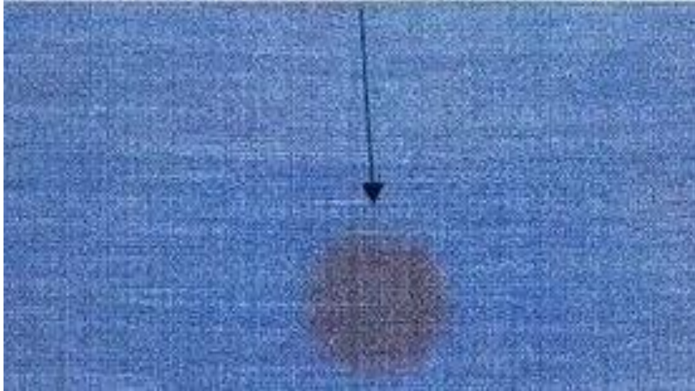
Fig 2.7: Oil spot Remedies: Correct machine support
