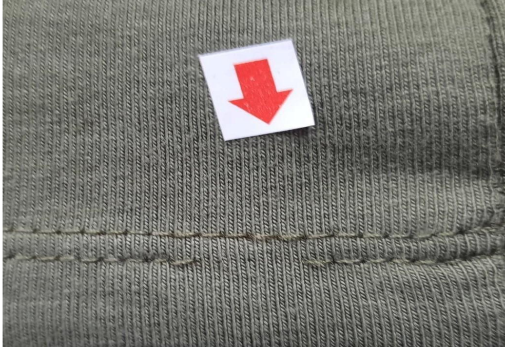
Fig 2.6: Needle thread breakage.
