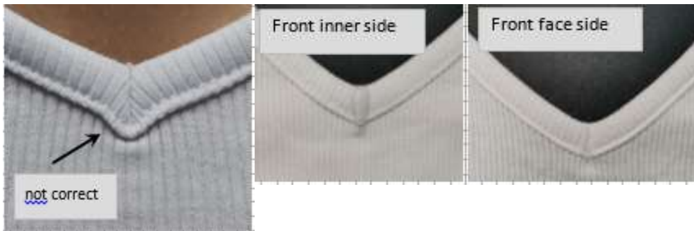
Figure: 3. 74 Inner and Face side Piping
