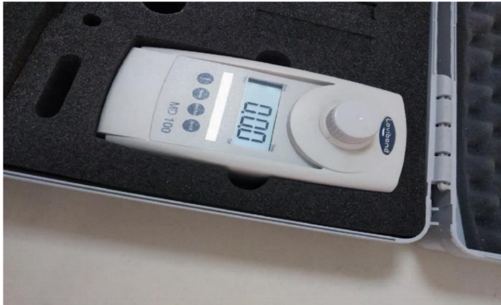
Figure: 3. 3 Suspended solid measuring instrument
