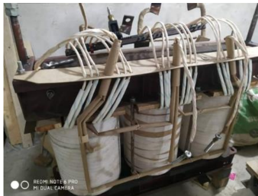
Fig: HT, LT Coil & Tap Changer.
