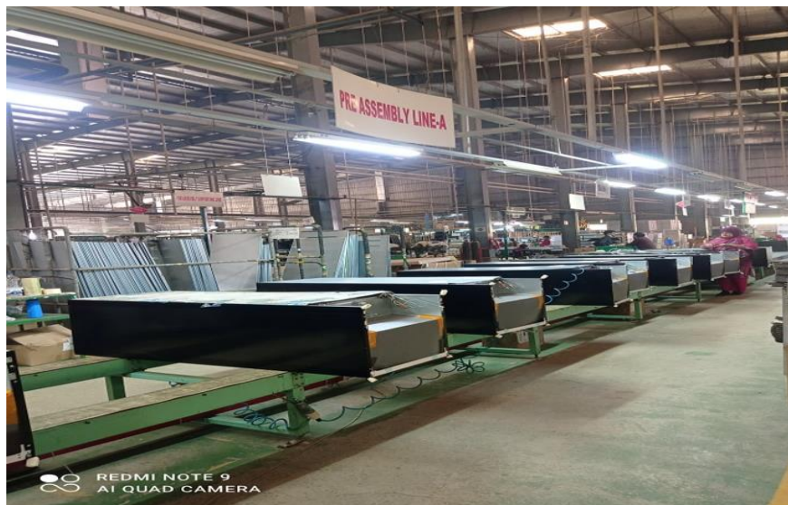
Fig 3.10: Pre-assembly line Refrigerator
