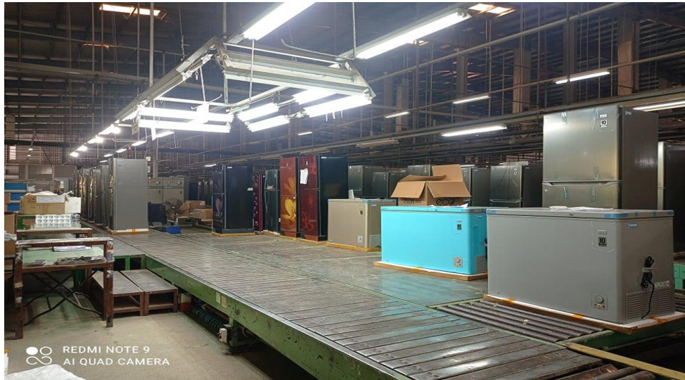
Fig 4.7: Final inspection section
