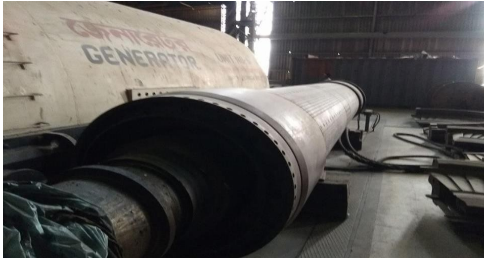
Fig. 5.4. Rotor of generator at GPS
