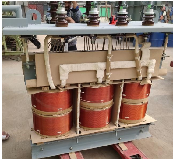
Fig 4.3,4 Transformer Copper Winding and Tank
