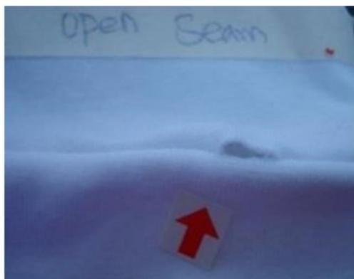
Picture 2: **Open seam or broken seam**
