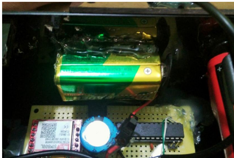
Figure 8.2: Implementation of Power Supply.
