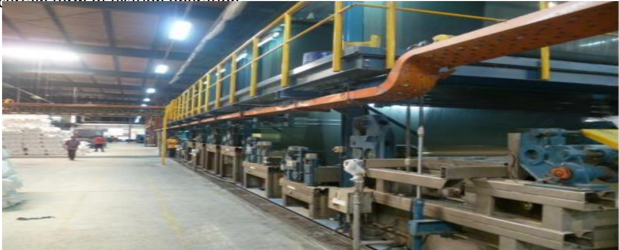
Figure: Beninger slasher dyeing and sizing machine1 in Shasha Denims Ltd.
