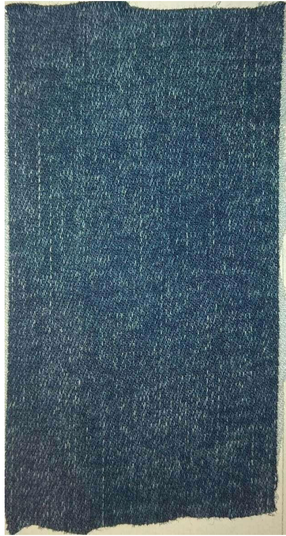
Fig3.4.4: After Stone acid wash
