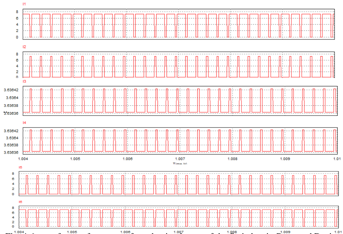
Fig. 4.6 waveforms of currents of conduction losses of the Switches in Proposed Design.
