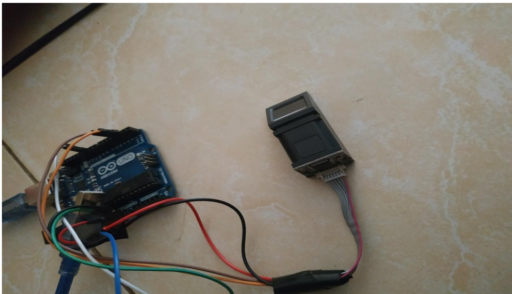
Figure 4.1.1: Fingerprint scanner with Arduino
