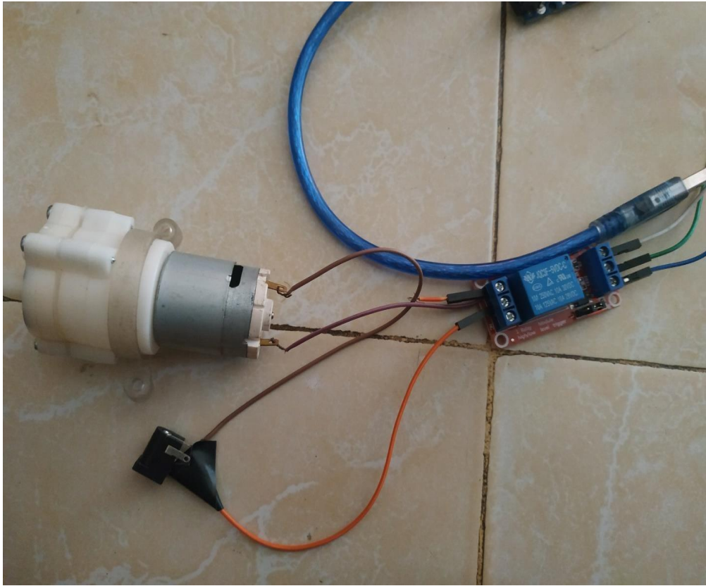
Figure 4.1.4: Connection between pump and relay module
