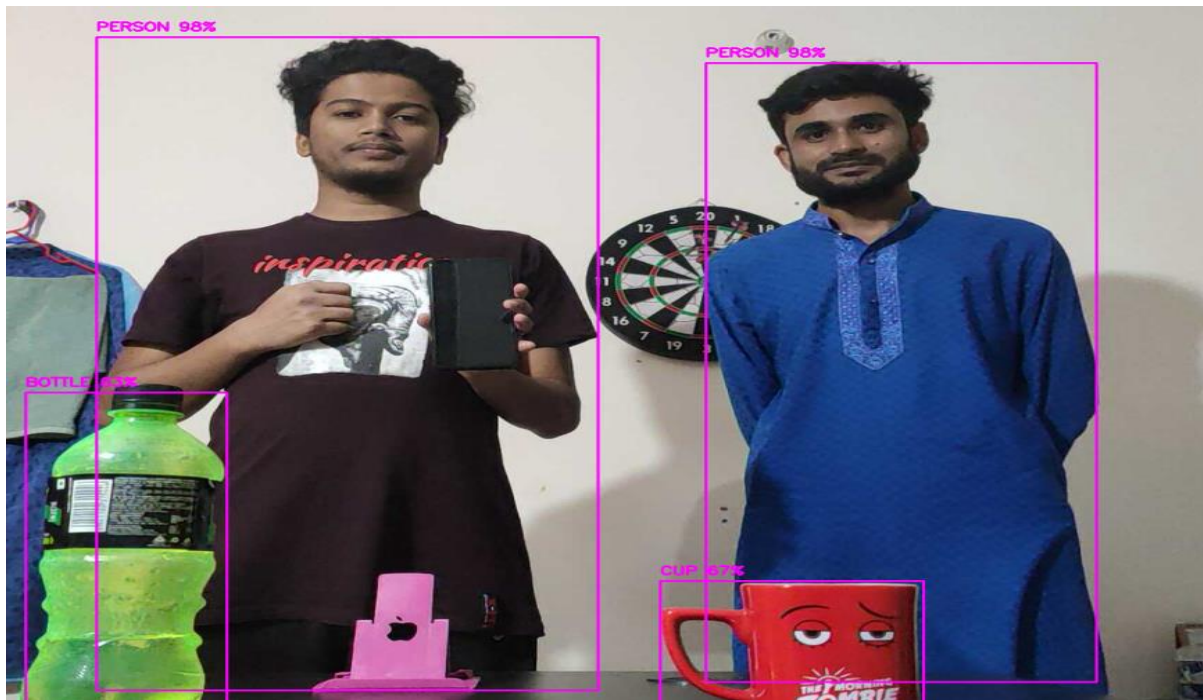
Figure 4.2.1: Detection and recognition of objects with goods.
