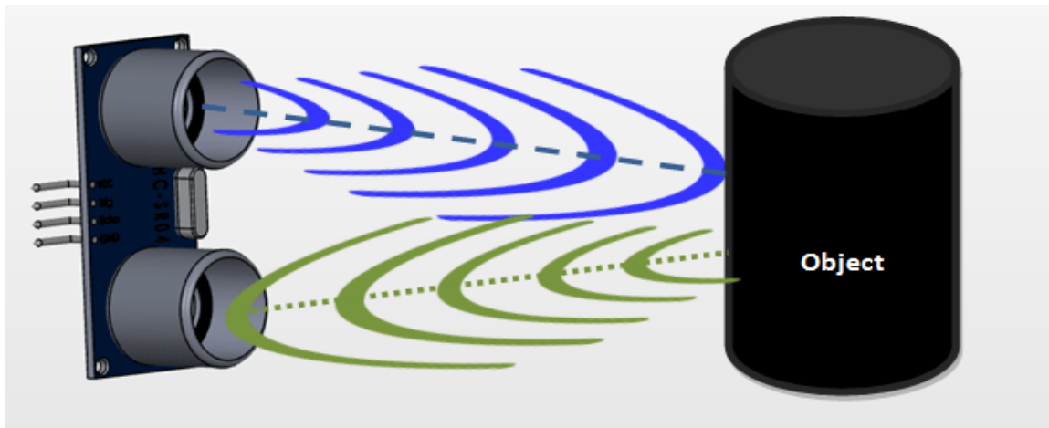
Figure 3.4.6: Mechanism of measuring the distance of Ultrasonic.
