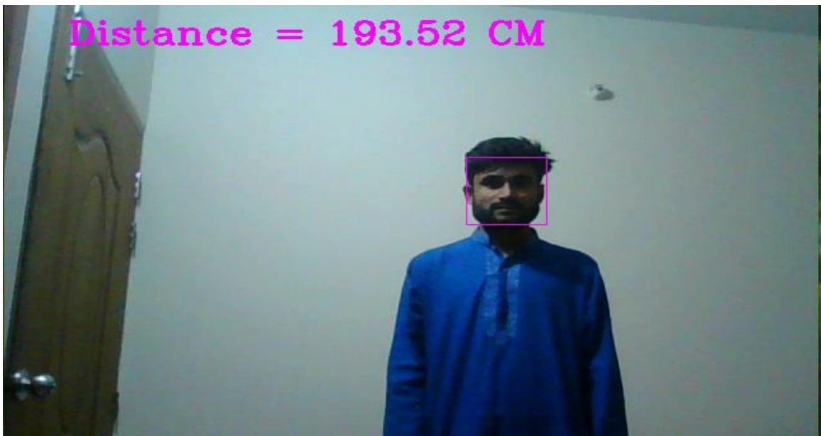
Figure 4.2.7: Distance Measurement using Focal Length of Person.
