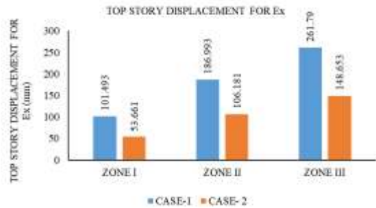
Fig. 6. Top story displacement for seismic load (mm)
