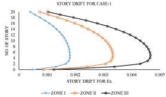
Fig. 7. Story drift for seismic load: case-1
