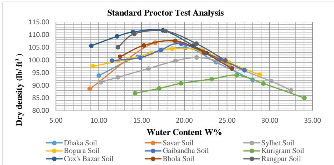
Fig. 4: Standard proctor test analysis for all soil samples.
