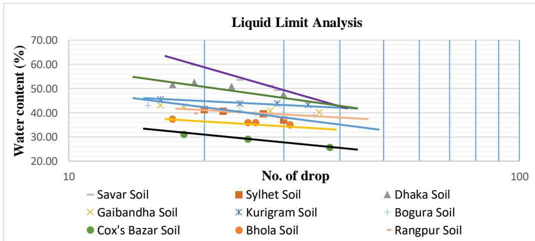
Fig. 3: Liquid limit analysis for all soil samples.
