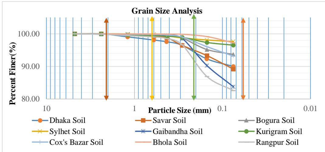
Fig. 2: Grain size analysis for all soil samples.
