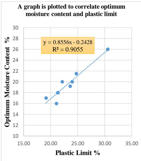
The linear equation graph is shown in figure 5, where 'y' is denoted as OMC and 'x' is denoted as PL. The correlation coefficient is denoted by the letter 'R'. When the plastic limit value is put into this equation, the new results of OMC are visible. It is well known that R-value near 1 indicates a strong correlation. For this research the result of  $y = 0.8556x - 0.2428$  and  $R^2 = 0.9055$  in this case.
